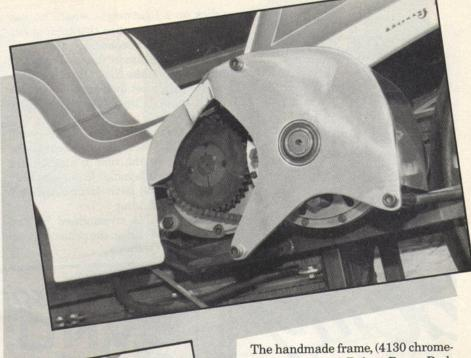
moly) contains 16 Pulsar Power Pack Batteries, imported by McNeil Motorsports, of Santa Ana, CA. These are the sole energy source used to spin that Prestolite Electric Motor (a real "motor"cycle). The throttle control is a pulse width modulation device that, even when explained in detail, was a bit too complicated for me. I did understand that the motor is sent pulses of electrical energy, at a rate of 2 khz, the pulse width being varied by the rider (hand throttle) as needed.
